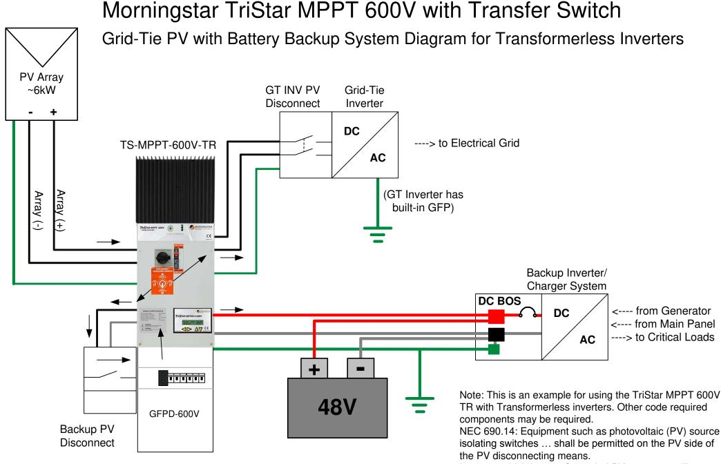
Inverters which have a Grounded PV array can utilize a single-pole switch before the TriStar MPPT 600V TR as a single PV system disconnect.
