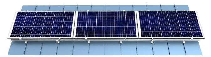
These pre-assembled Mid Clamps have a unique T-Bolt locking feature that ensure the T-Bolt remains vertical and in full contact with the rail to eliminate pull out. The spring-loaded top clamp and open collar nut accommodates module frames from 31 to 50 mm. The added Loctite easily engages the T-Bolt from the top of the collar nut. The shared rail adaptor converts standard rail to shared rail to allow landscape mounting of PV panels on E-W rails.
