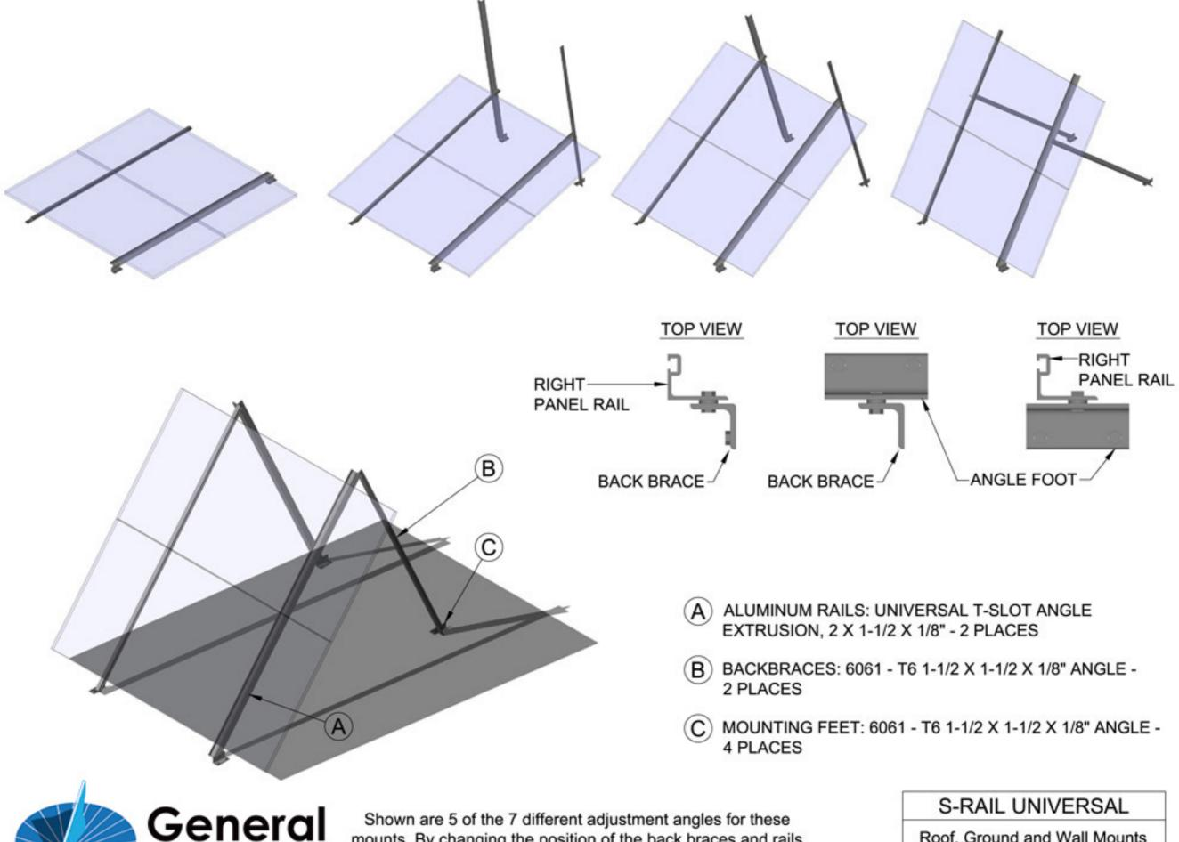
Shown are 5 of the 7 different adjustment angles for these mounts. By changing the position of the back braces and rails you can move your array more vertical or horizontal.
