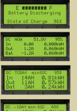
**Battery Status Screen** - Easily see your system's current condition with this at-a-glance display. This screen shows an easy to interpret "fuel gauge" style status bar, current state-of-charge and whether you are currently charging or discharging your batteries. This is useful for those system owners who want a way to quickly understand the current state of their battery bank.
