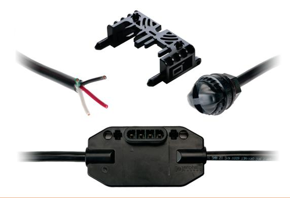
The **Engage™ Cable** is a continuous length of 12AWG cable with pre-installed connectors for Enphase Microinverters. The cable is handled like standard outdoor-rated electrical wire, allowing it to be cut, spliced and extended as needed.
