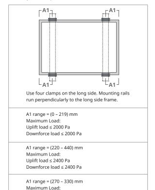
Uplift load ≤ 2400 Pa Downforce load ≤ 5400 Pa
