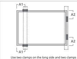
Use two clamps on the long side and two clamps on the short side.
