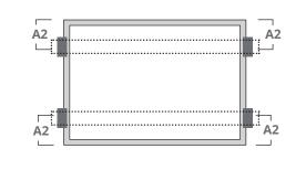
Use four clamps on the short side. Mounting rails run parallel to the long side frame.
