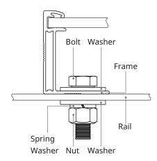
Modules should be bolted at the following hole locations depending on the configuration and loads:
