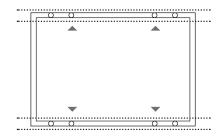
Maximum Load: Uplift load ≤ 2400 Pa Downforce load ≤4000 Pa
