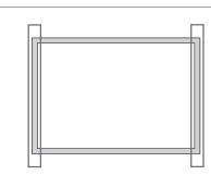
Use two insertion profiles running perpendicularly to the long side frame.
