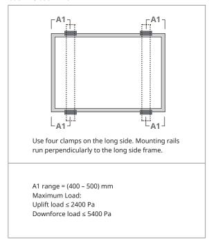
Rail-less clamping for CS3K-P, CS3K-MS, CS6K-P, CS6K-M, CS6K-MS, CS1K-MS, CS1H-MS
