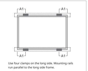
A1 range = (240 - 330) mm Maximum Load: Uplift load ≤ 2400 Pa Downforce load ≤ 4000 Pa
