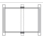
Use two insertion profiles running perpendicularly to the long side frame. An additional support bar should be placed below the module. Use two clamps on the support bar.
