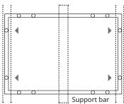
Maximum Load: Uplift load ≤ 2400 Pa Downforce load ≤ 5400 Pa
