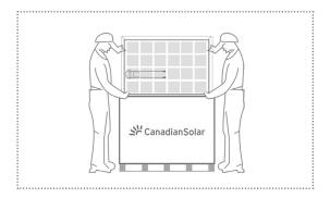
Do not stand, step, walk and / or jump on modules under any circumstances. Localized heavy loads may cause severe micro-cracks at cell level, which in turn may compromise module reliability and void Canadian Solar Inc's warranty.
